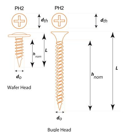
The FFX Dry Wall Screw is a case hardened Drywall Screw. It features a Twin Thread for increased pull out loading. The Bugle Head helps to prevent damage to the finished surface. The Sharp 25° point also avoids pre-drilling into Metals. The Wafer Head creates a large clamp down area when stitching drywall track or ceiling track together. A designed point avoids pre-drilling into Metals..
